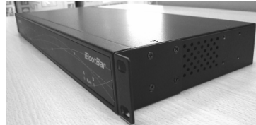
Installed R bracket:
