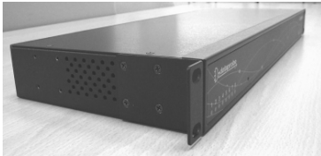
Installed L bracket:
