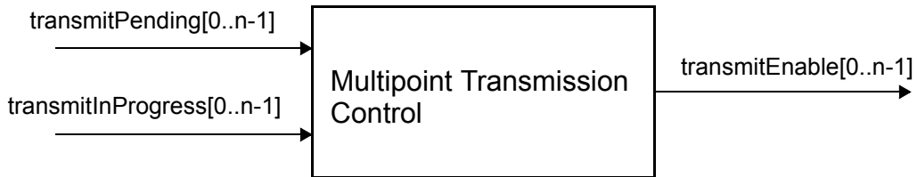
Figure 64-5—Multipoint Transmission Control Service Interfaces
