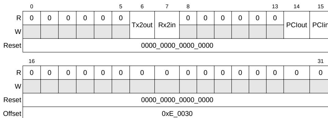
Figure 18-7. General-Purpose I/O Control Register (GPIOCR)
