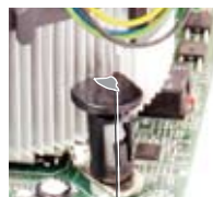
Narrow end of the groove points outward
